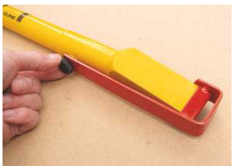
A steel guard is screwed to the tool side
